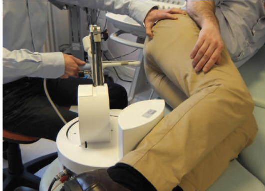
Fig. 6.9 The 6-DOFs Apollo robot assisting an urologist who comanipulates an endorectal ultrasound probe with virtual fixtures constraints, (Vitrani et al., 2017). © ISIR.
